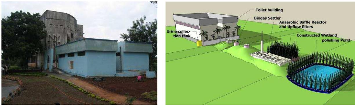
**Fig 3.** Low-flush pour-flush urine diversion toilets at Adarsh Vidya Mandir school (source: ESF). Left: New toilet centre in 2008; right: technical drawing of sanitation system of the school.
