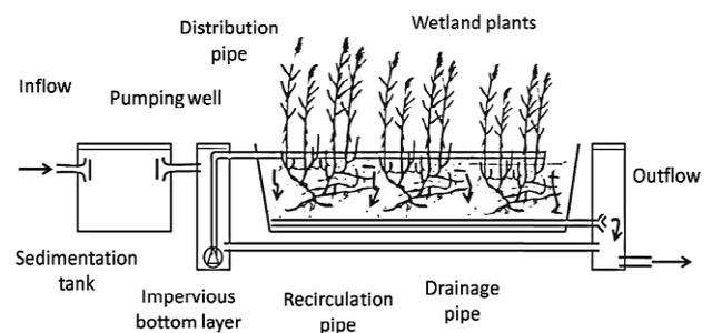
**Fig. 8:** Schematic structure of vertical flow reed bed (source: Brix and Arias, 2005)<sup>4</sup>.
