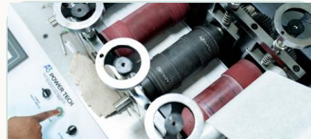
09 Emboss and seal the pad
