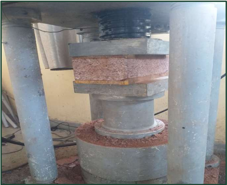
Compressive strength testing, ADSWE materials lab
