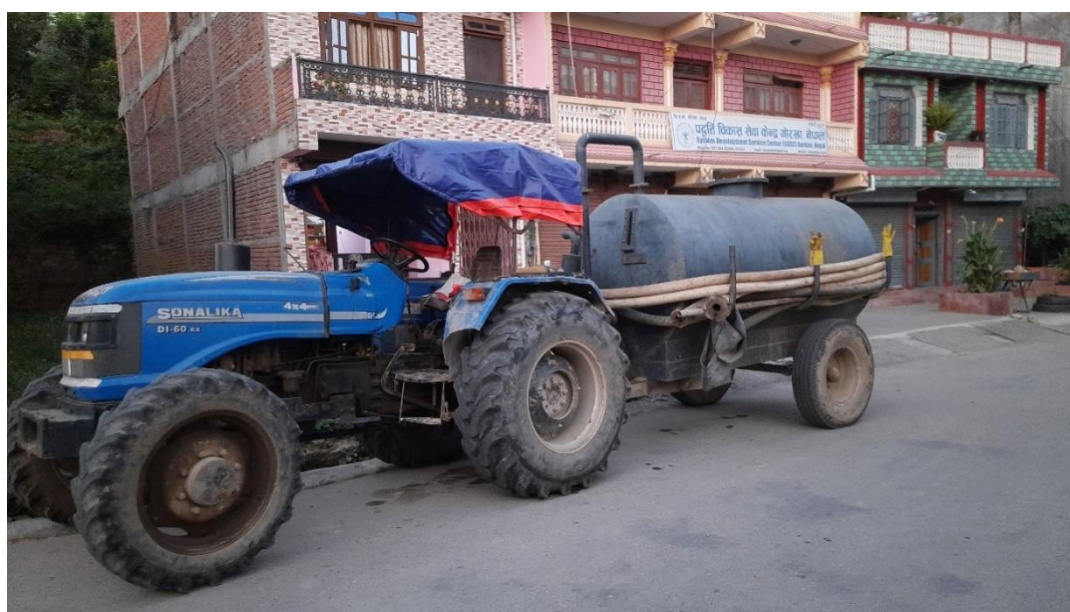
Figure 11: The desludging vehicle.
