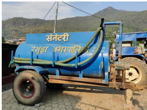
Figure 13: The desludging vehicle owned by Resunga Municipality.
