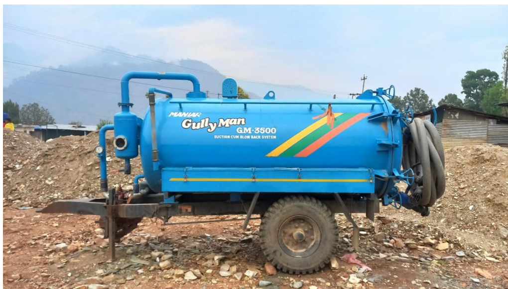
Figure 8: Compartment of vehicle for desludging service that is assembled with tractor.
