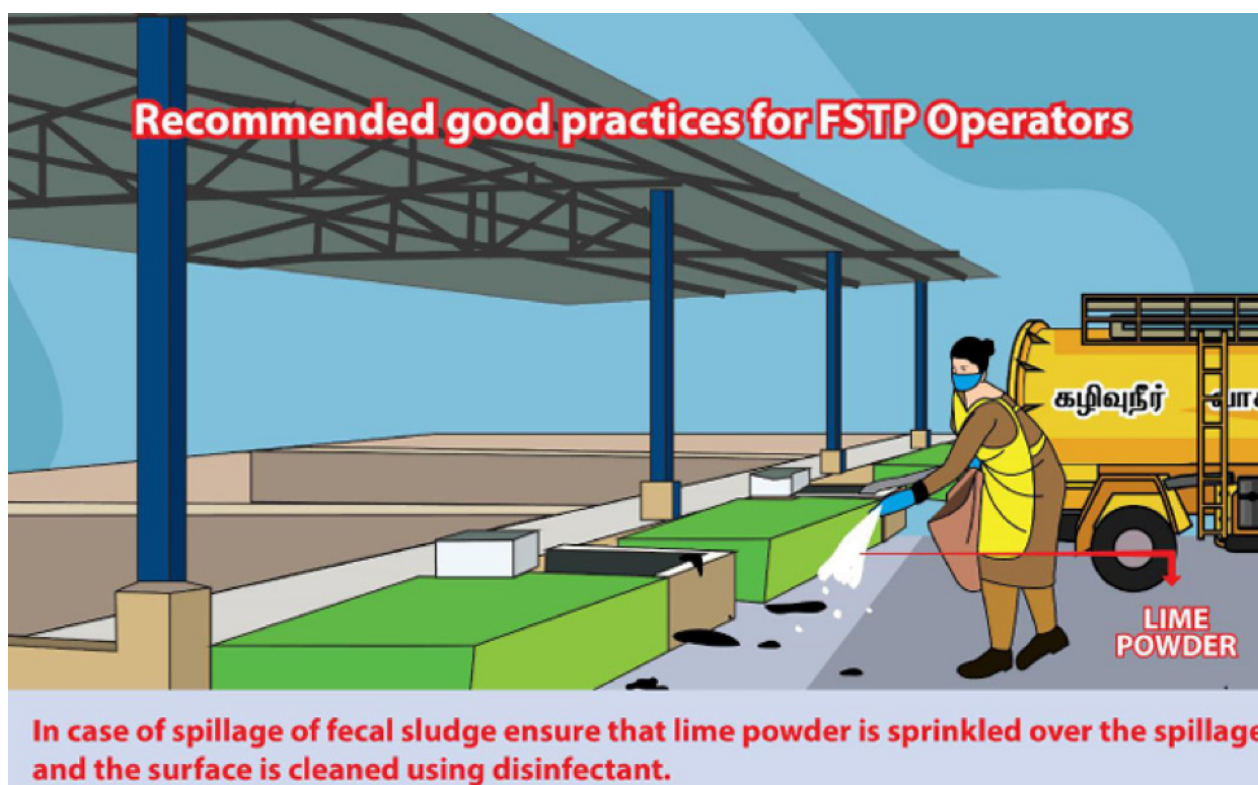
Figure 36. Protocol for management of spillages at site
