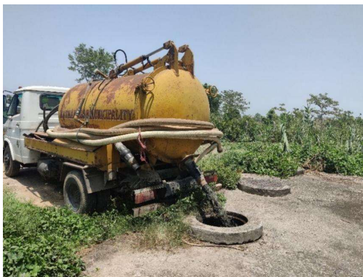
Figure 17: FS disposal in WWTP by municipal desludging vehicle.
