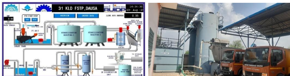
Figure 6: Septage Treatment Procedure and MBBR tank at FSTP Plant. (Source: Rajat, Ravie. CFAR. 2025).
