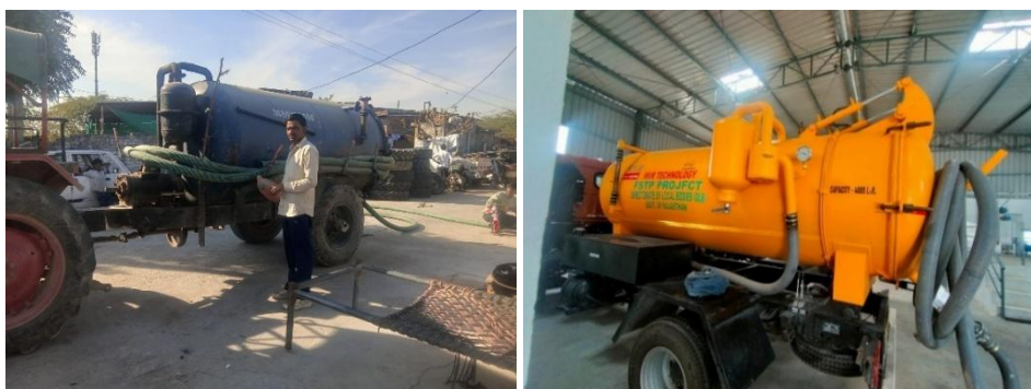
Figure 7: Cesspool vehicles (Private and FSTP owned) used for emptying and transportation. (Source: Madhu, CFAR. 2025).
