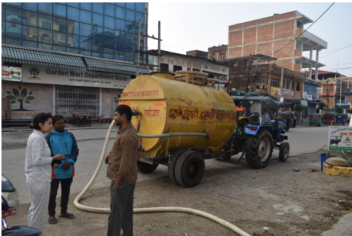
Figure 8: Mechanical Emptying of Containments in Triyuga Municipality.
