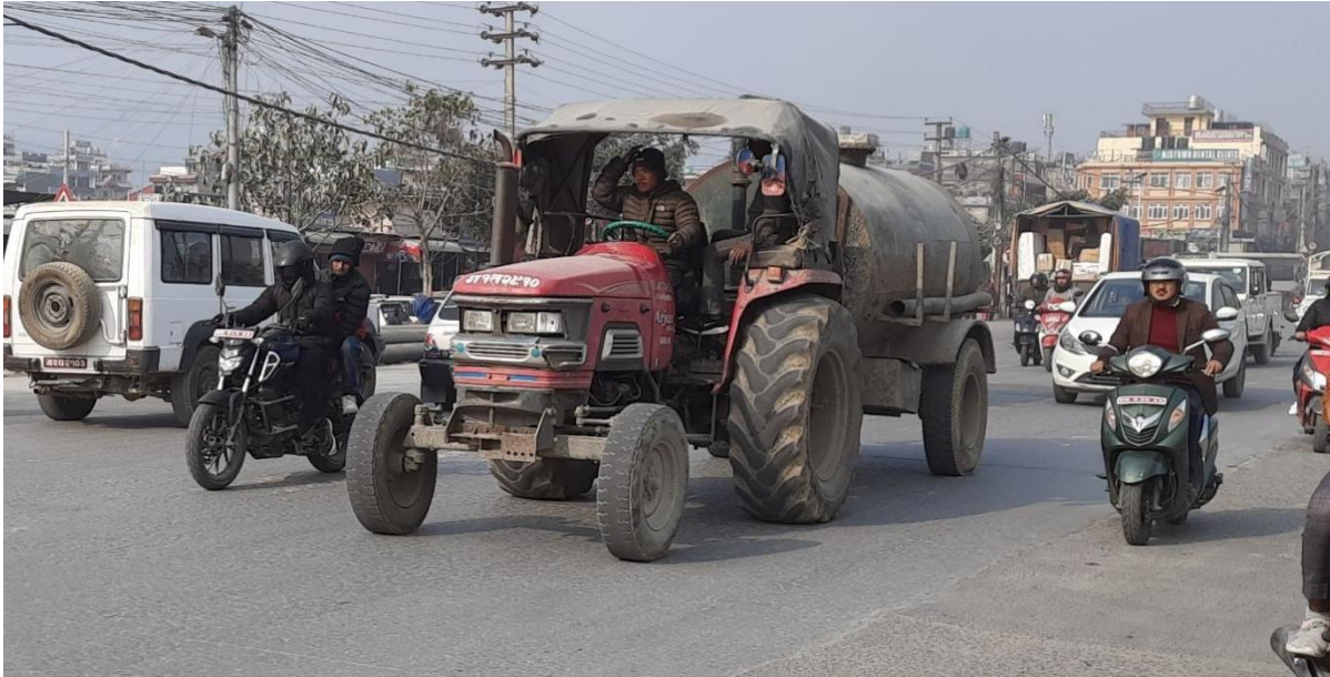
Figure 8: Mechanical Desludging Vehicle available in Pokhara Metropolitan City.
