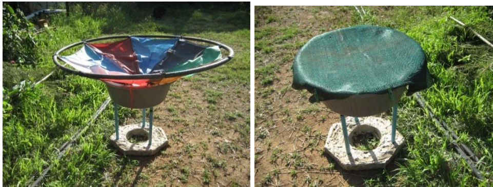
Smaller “rain catchers” developed good quality water but in limited amounts. 0.9litres per mm rain
