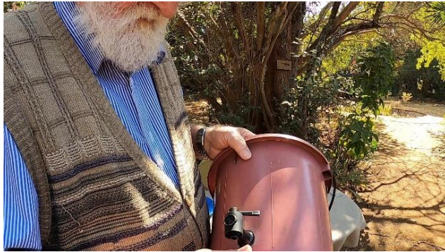
Photos take from video reveal how important it is to get a good watertight seal between the filter and the bucket base. Rubber seals are used make the crucial joint watertight.
