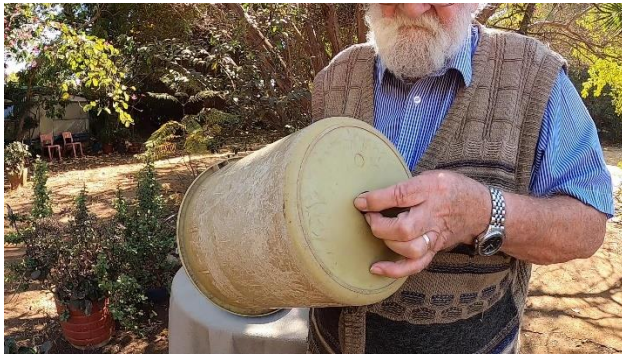
Photos take from video reveal how important it is to get a good watertight seal between the filter and the bucket base. Rubber seals are used make the crucial joint watertight.
