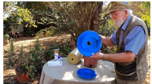
Photos take from video reveal how important it is to get a good watertight seal between the filter and the bucket base. Rubber seals are used make the crucial joint watertight.
