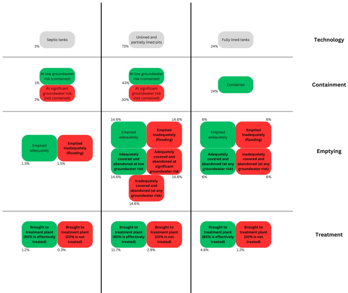
Figure 4: Sanitation containments and their fate with the respective amount. Boxes marked in bold are endpoints. Boxes marked in green and red are considered safely, respectively unsafely managed.
