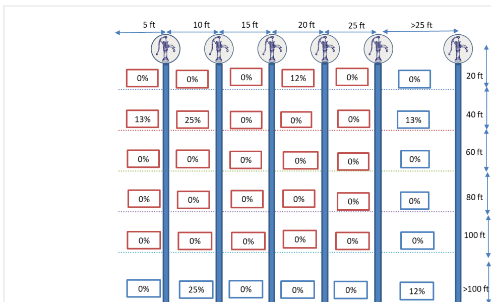
Figure 16: Depth of hand pumps and tubewells and lateral spacing of it with containment types lined pit with semi-permeable walls and open bottom.
