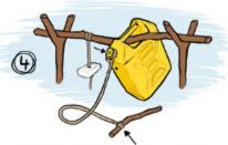
ASSEMBLE THE TIPPY TAP AS SHOWN IN THE PICTURE. ATTACH ONE END OF THE STRING TO THE CAP OF THE JERRY CAN AND THE OTHER END TO AN ~50 CM LONG STICK.
