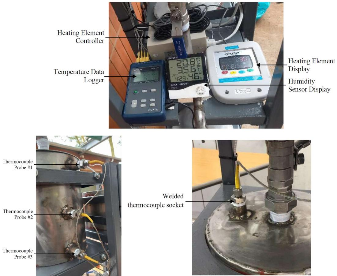
Figure 5.4. Installation of the sensors
