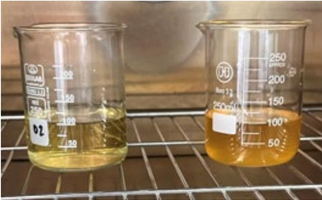
**Figure 2.2. Stabilised (right) and hydrolysed (left) urine samples**
