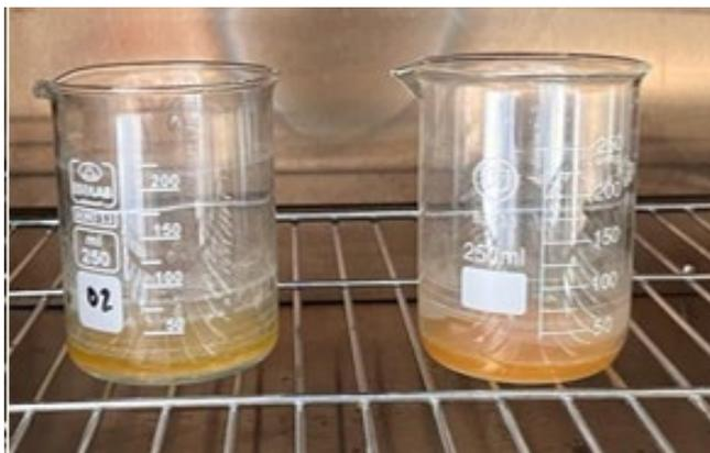
**Figure 2.3. Stabilised (right) and hydrolysed (left) urine samples at the after 5 days evaporation at 40°C**
