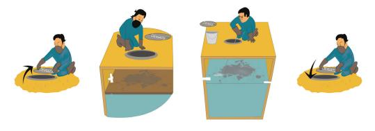
**b)** Also you can check the flow of wastewater in sewer lines by using of color, open all inspection chamber, mix the color powder with water and flush the water in to the closet and then check the flow in each inspection chamber until DEWATS if you see the color than there is flow if you don't see than there is blockage.
