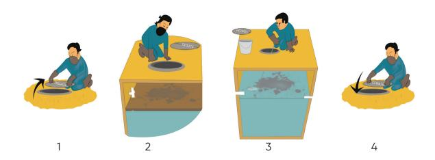
**4.** Once in a year check the sludge level in Settler using a wooden stick
