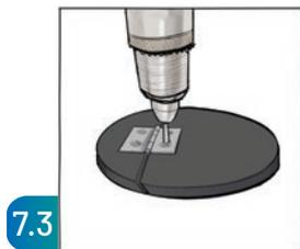
Drill holes with 4 mm bit for the rivets
