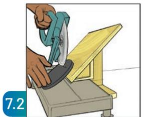
Cut at 3.5mm from one end at 50°-60° angle
