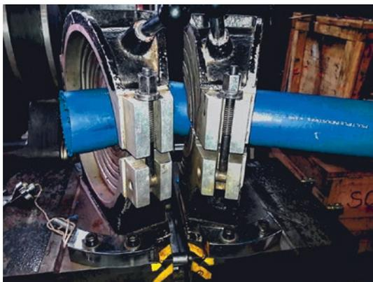
Joining shorter pipe to Main WASHaLOT pipe using SGH-315 fitting fusion welding machine at Multiple Industries (U) Ltd. (photo by C.Mukiibi)
