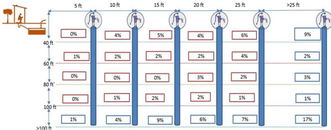
**Figure 12: Depth of hand pumps and lateral spacing of it with containment types lined pit with semi-permeable walls and open bottom.**
