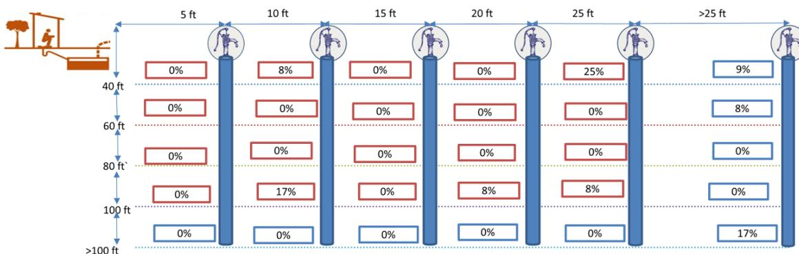
**Figure 13: Depth of hand pumps and lateral spacing of it with containment types lined tank with impermeable walls and open bottom.**
