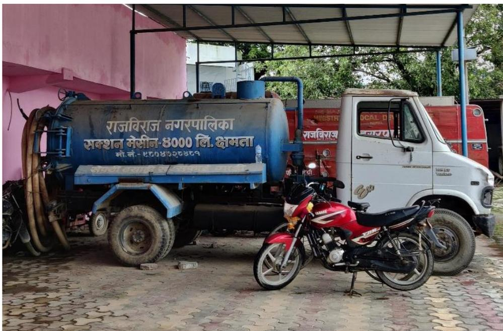
**Figure 11: Desludging suction truck of Rajbiraj Municipality.**
