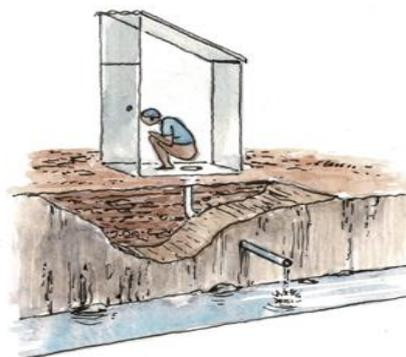
Figure 4: Toilet discharges directly to open drain.
