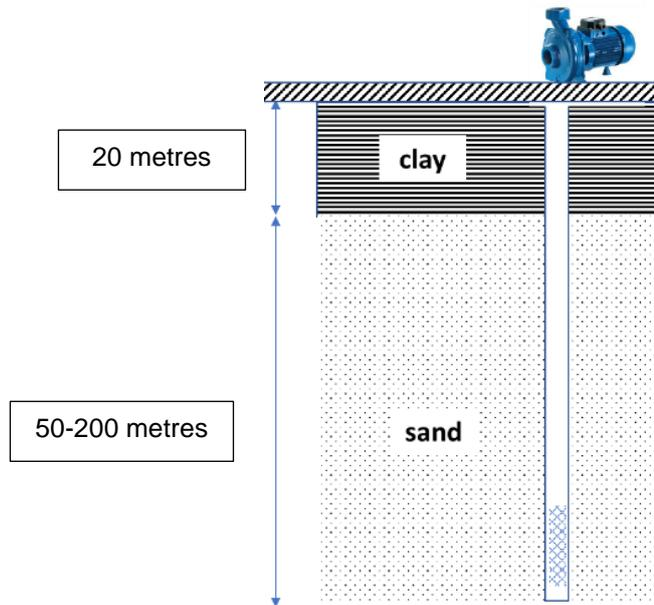
**Figure 9: Soil profile in Faridpur district and location of tube well screen.**
