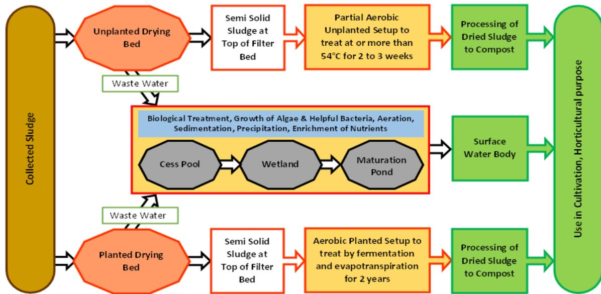
Figure 8: The treatment flow of the Faridpur FSTP.
