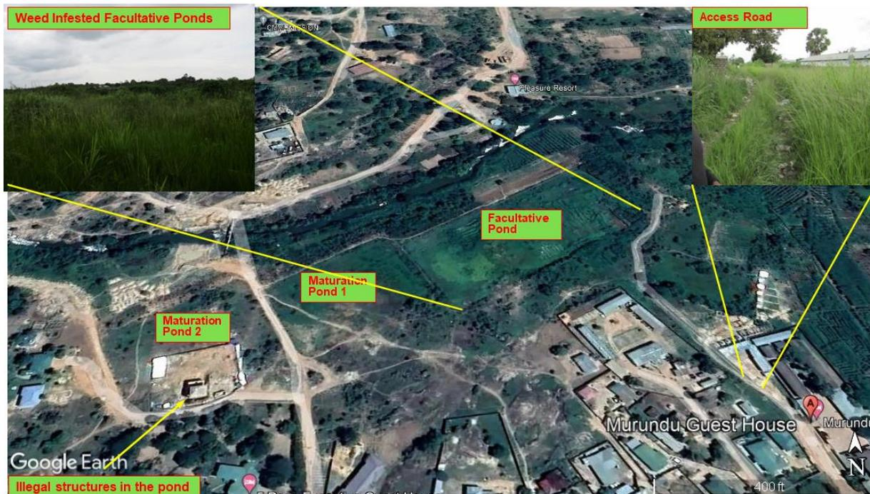
**Figure 6: The Suburbs WWSPs with inserts on state of the Access Road and the Weed Infested Facultative Pond (Source: Author).**
