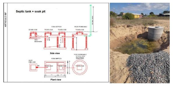
Figure 4: (Left): Sketch of the ordinance where the design of septic tanks is outlined; (Right): Septic tank under construction. Source: (D&A and EP, 2021).
