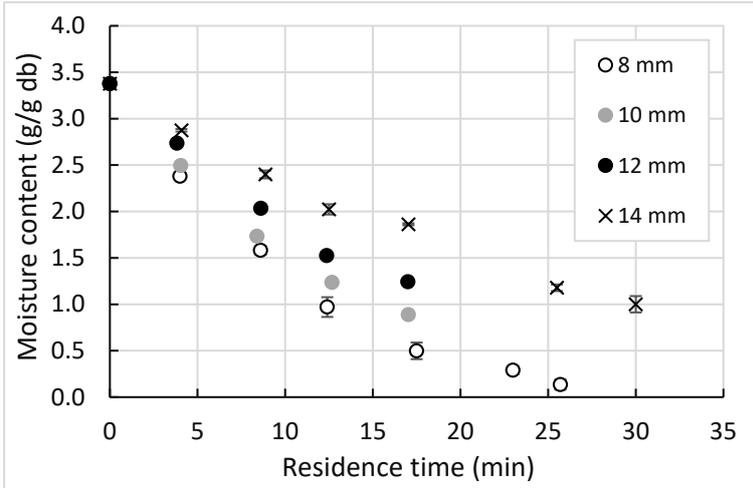
Moisture content versus residence time for the raw sludge, mixed with sawdust and pre-dried
