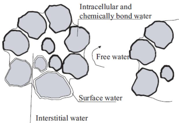
Figure 4. Different types of moisture in the sludge (Chen, Lock Yue and Mujumdar, 2002)
