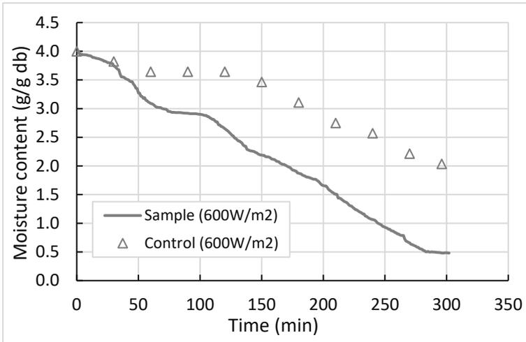
Moisture content versus time inside the solar drier and the control (sample placed at the open air) during overcast conditions
