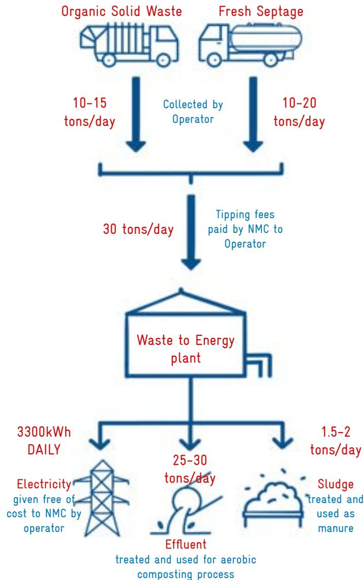
Schematic of the Waste to Energy Process
