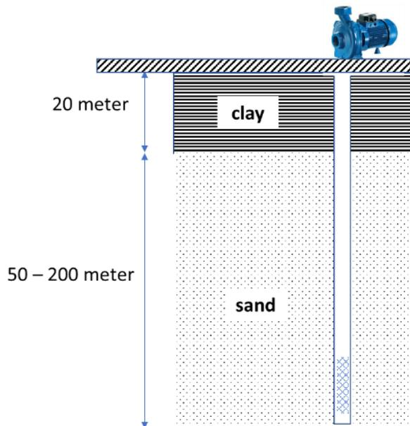
**Figure 7: Soil profile Nilphamari city and location of tube well screen.**
