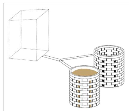
Figure 3 Twin pit system (eawag & IWA,
