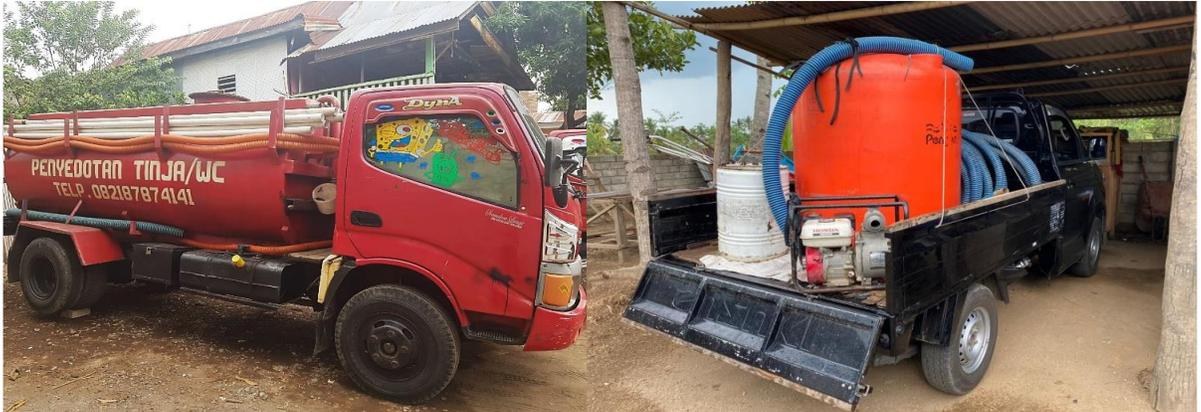
*Pit emptying service providers use a 6-wheel truck with steel tank as in Makassar City (left picture), and use a pick-up with fiberglass tanks as in Lombok Timur Regency.*
