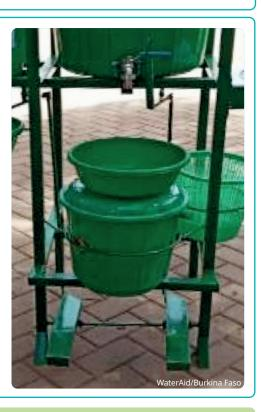
Another option for a foot-operated pedal, rather than using a rigid lever mechanism, is to operate the tap or soap dispenser using a small steel cable (e.g. bike brake cable), which may require less maintenance if the cable is of good quality and protected against corrosion. This is illustrated in Figure 7.
