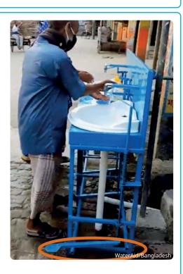
▲ A pedal arrangement working in an upward direction. Note the lift cock is getting direct upward push for water distancing.
