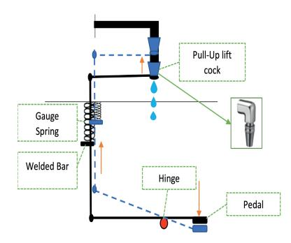
▲ Mechanism 2: Pedal arrangement for pull-up lift cock.
