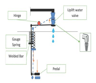
▲ Mechanism 3: Pedal arrangement for pull-up lift cock.
