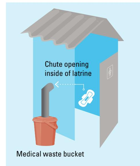
ii. This method is not appropriate in all settings. It is only appropriate if there are direct-drop pit latrines that are not connected to a septic system, and will be appropriately decommissioned.
