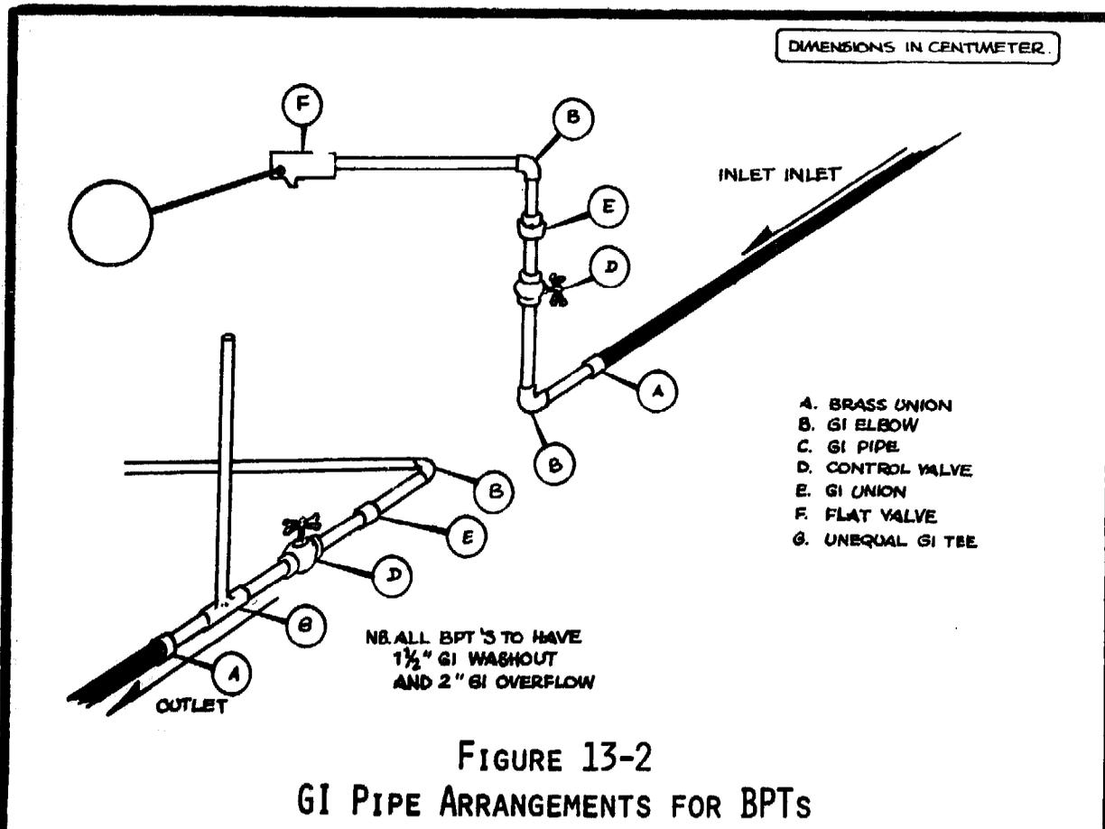
Inner dimensions: Must be large enough to accommodate the fittings which will be installed. Minimum width = 40cm; minimum length = 40 cm (80cm if a float valve is to be installed), and depth to be 50cm. Can be adjusted to accommodate dimensions of CGS roofing.
