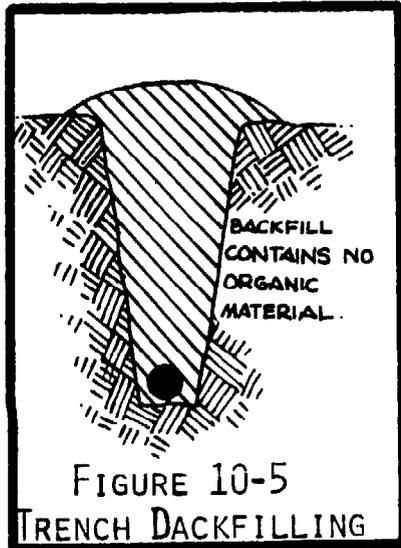
The pipeline should be fully buried except for a three-meter section at each joint. This joint section should only be about half-buried until the pipeline has been filled with water and allowed to stand at full static pressure for 24 hours. This makes it very easy to locate leaking joints, since water will have seeped up to the surface within that time. Once all joints have been tested, they can be fully buried.
