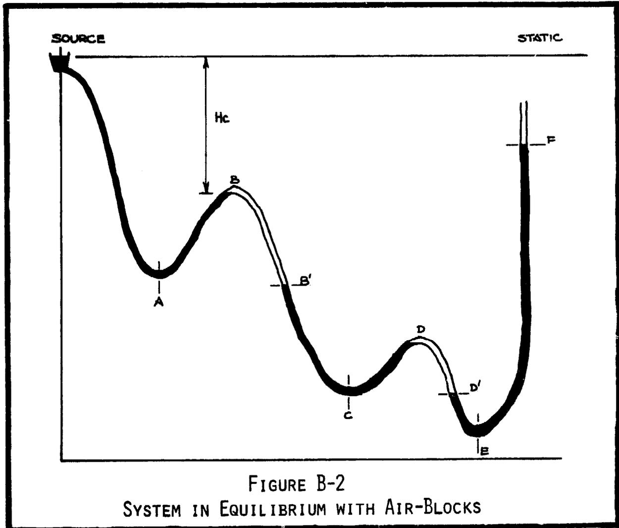
The head between the source and top of the first air-block shall be called the compression head,  $H_c$ ; the sections of pipe containing the initial, uncompressed volumes of trapped air shall be the critical sections (sections BC and DE in Figure B-2); the top of an air-block will be the high point (points B and D); the bottom of an air-block will be the low point (points B' and D'); and the height to which the water will rise shall be called the maximum elevation (point F).
