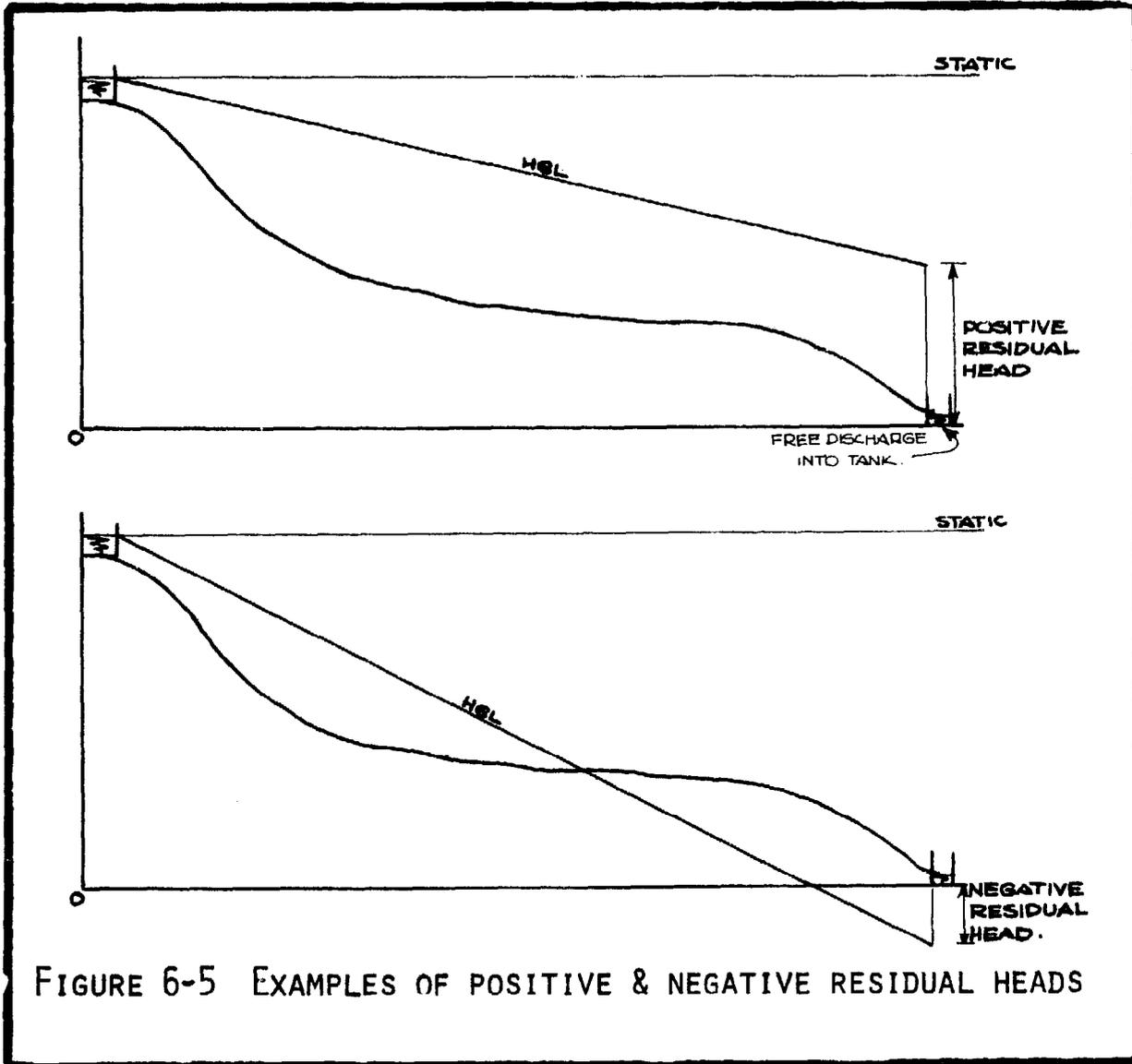
FIGURE 6-5 EXAMPLES OF POSITIVE & NEGATIVE RESIDUAL HEADS
