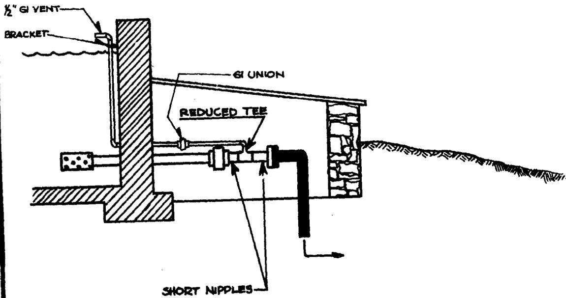
FIGURE 11-6 TYPICAL OUTLET PIPING
