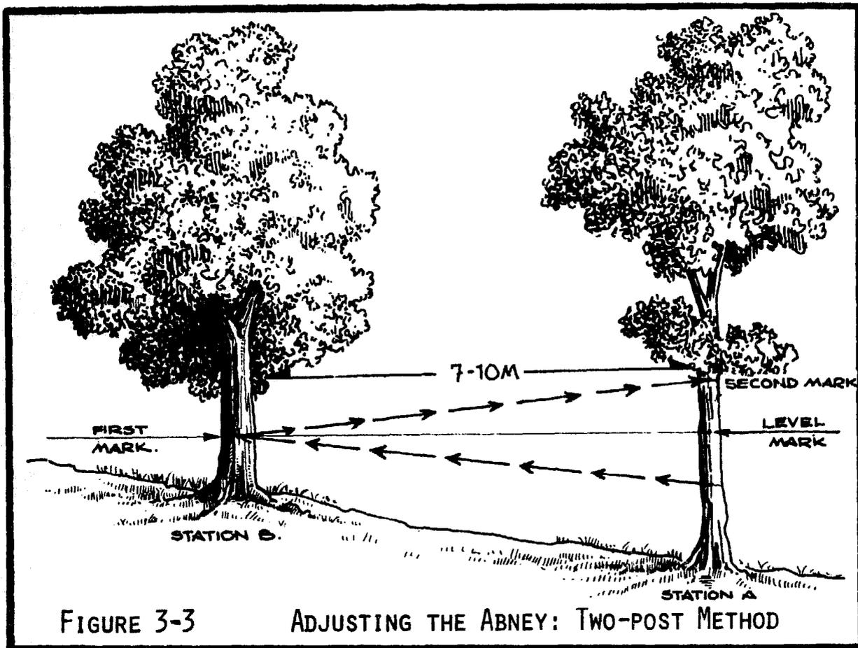
FIGURE 3-3 ADJUSTING THE ABNEY: TWO-POST METHOD
