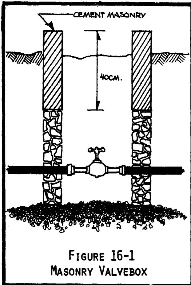
cemented into the walls of the box, and the box should be built on a bed of gravel or crushed stone several centimeters deep to allow quick drainage of leakage or moisture. Refer to Figure 16-1.
