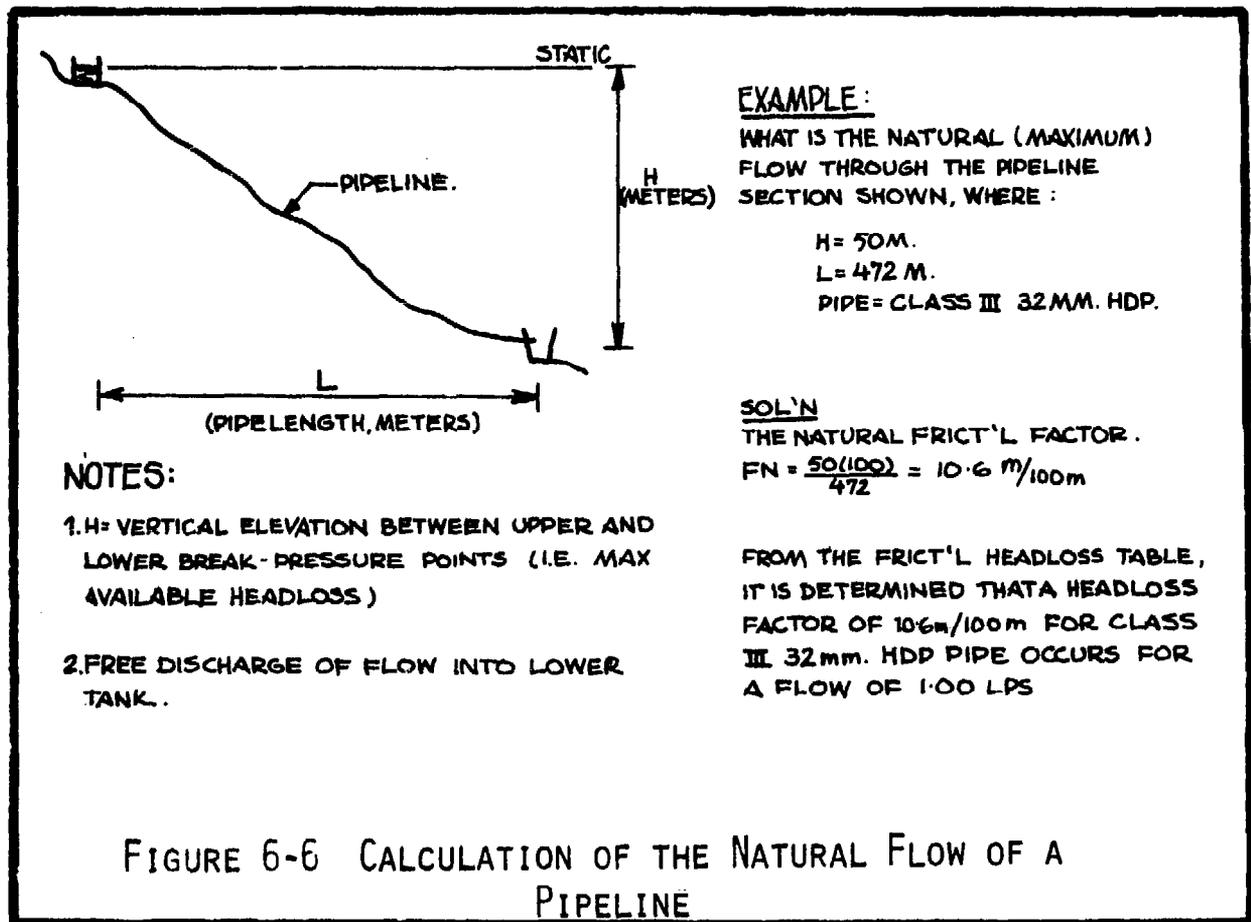
If the natural flow of a pipeline is greater than the safe yield, then the pipe will drain faster than it can be filled, and the result will be that the pipe will not flow full. In such a case, the HGL will lie on the surface of the water inside the pipe. A non-full flowing pipe is not under any pressure (except where the pipe flows full in U-profiles). If there are no tapstands located along a pipeline section that is not flowing full, then this is of no consequence.
