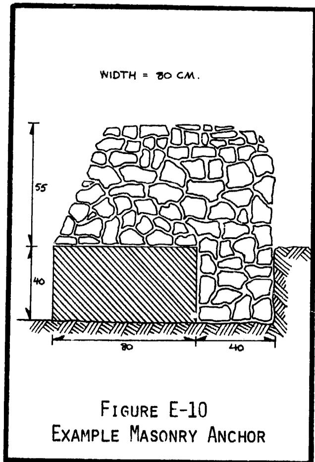
Designing the masonry block anchor (east bank)
