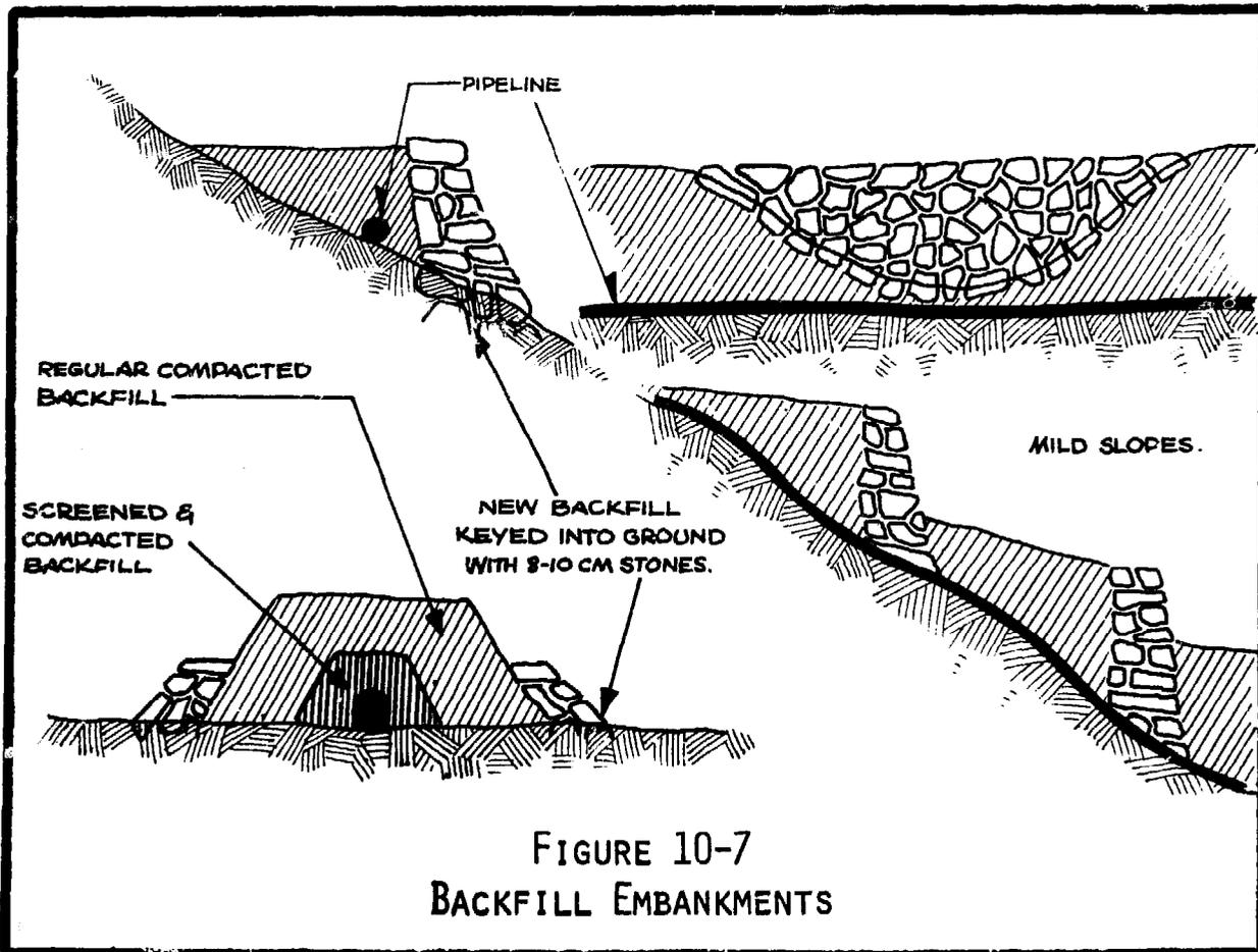
Steep slopes: Where the trench cuts down a steep incline, the backfill is vulnerable to easy erosion by rainfall, which will tend to wash all backfill to the bottom of the slope. Facing the trench with stone, as shown in Figure 10-8, will help to protect the backfill.
