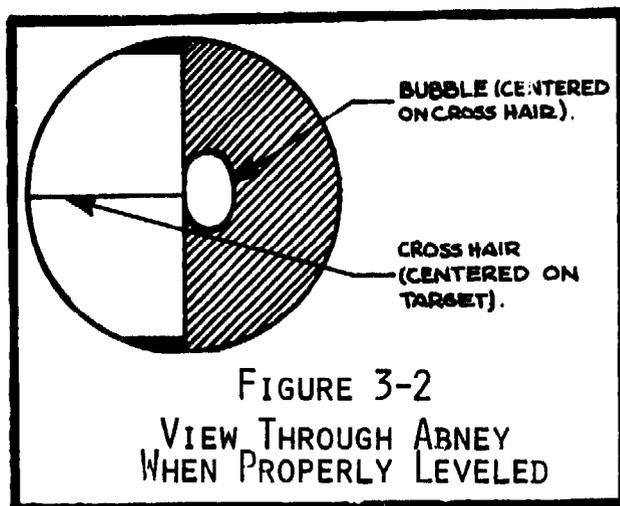
all aligned horizontally, as shown in Figure 3-2. The angle of view (technically known as the vertical angle) is then read on the arc in degrees.
