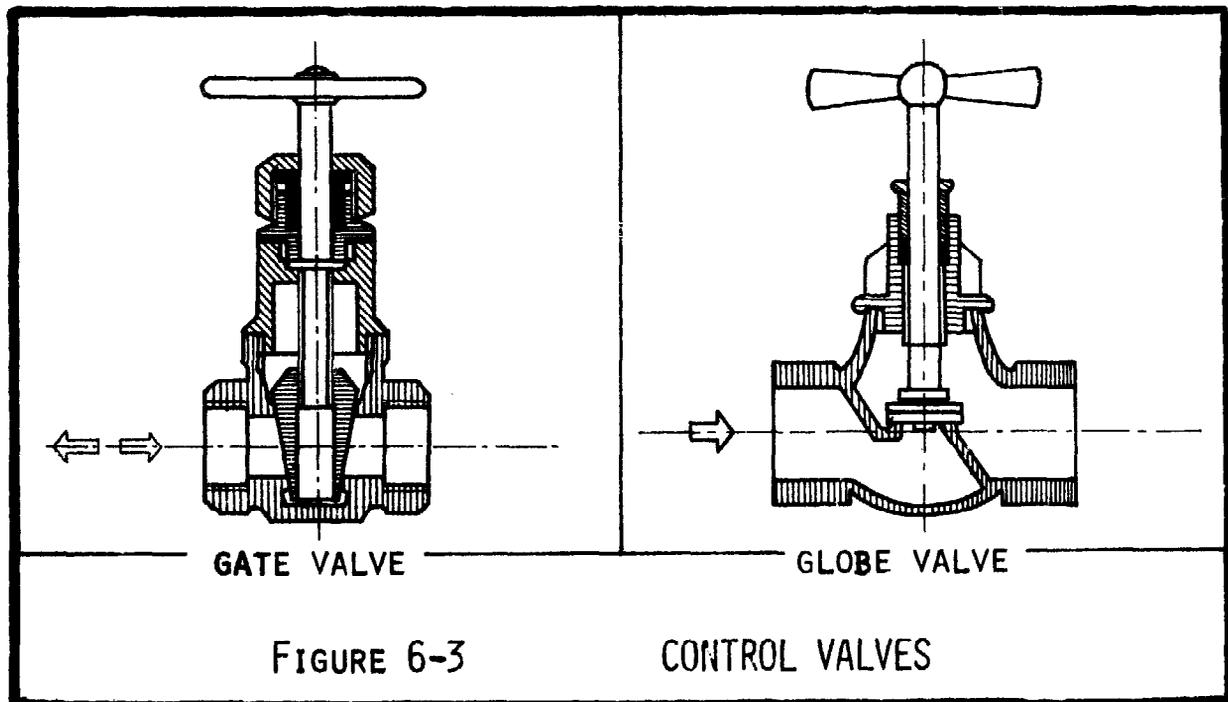
Gate valves: Gate valves serve as on/off control valves, for the purpose of completely cutting off the flow. Generally, they are located at the outlets of intakes, reservoirs, strategic break-pressure tanks, and at major branchpoints. They are not recommended for use in regulating flow (ie- partially open or closed) since the water will erode the bottom edge of the gate and result in a leaky valve whenever it is meant to be closed. Direction of flow through the valve is unimportant.
