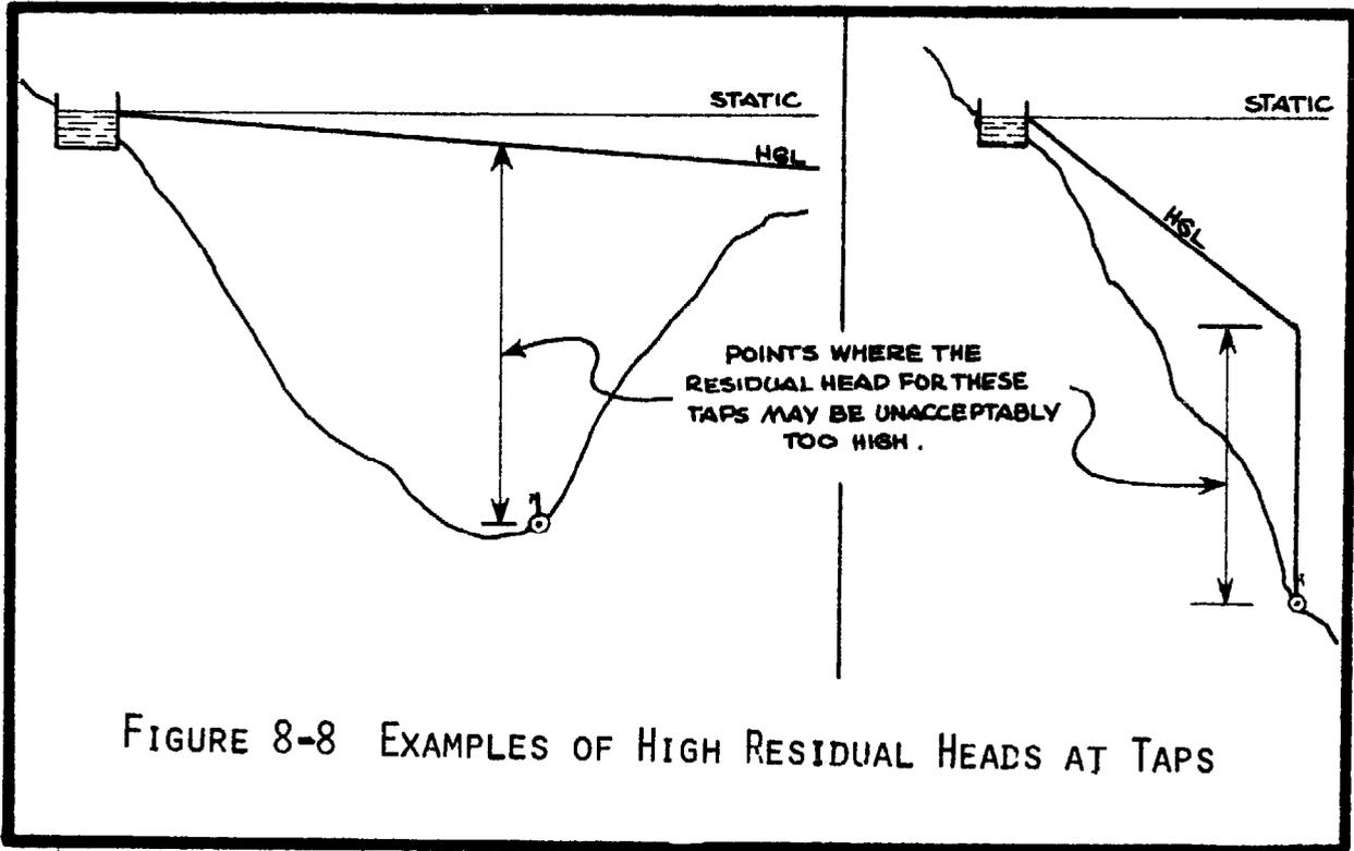
For such cases, it is possible to install a device which creates high frictional losses in only a short length of pipeline. This sort of frictional diffuser can be easily manufactured in the field, using HDP pipe and fittings. A design for this is shown on the next page.
