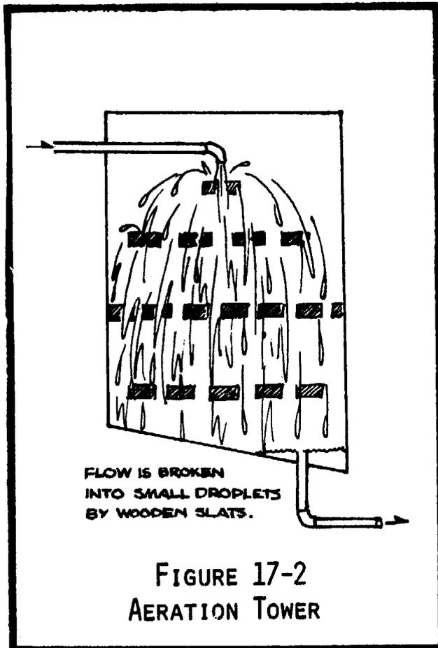
The easiest method of aeration is to build a tower, as shown in Figure 17-2, which has several tiers of plastic screens or wooden slats. These mechanically break the water flow into small droplets, which, because of their increased surface area, can absorb oxygen quicker. Such a tower can be built as part of a sedimentation tank or collection tank, or even the reservoir.
