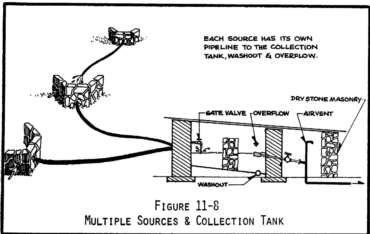
by the distances and elevations between the sources. Flow from higher sources can be piped directly into lower sources, or each source may have its own individual pipeline to a single collection tank or
