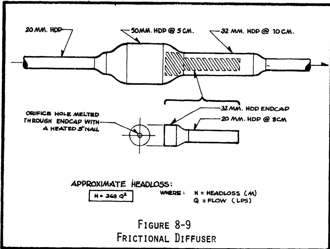
The orifice in the endcap is made using a hot 3" nail to melt a hole. For a flow of 0.225 LPS, this diffuser will create approximately 20-25 meters of headloss. Adding more holes decreases the headloss; if the headloss of a single diffuser is not enough, add a second one. The pipe section must be of Class IV HDP if the diffuser will be subjected to a static pressure greater than 60 meters of head.
