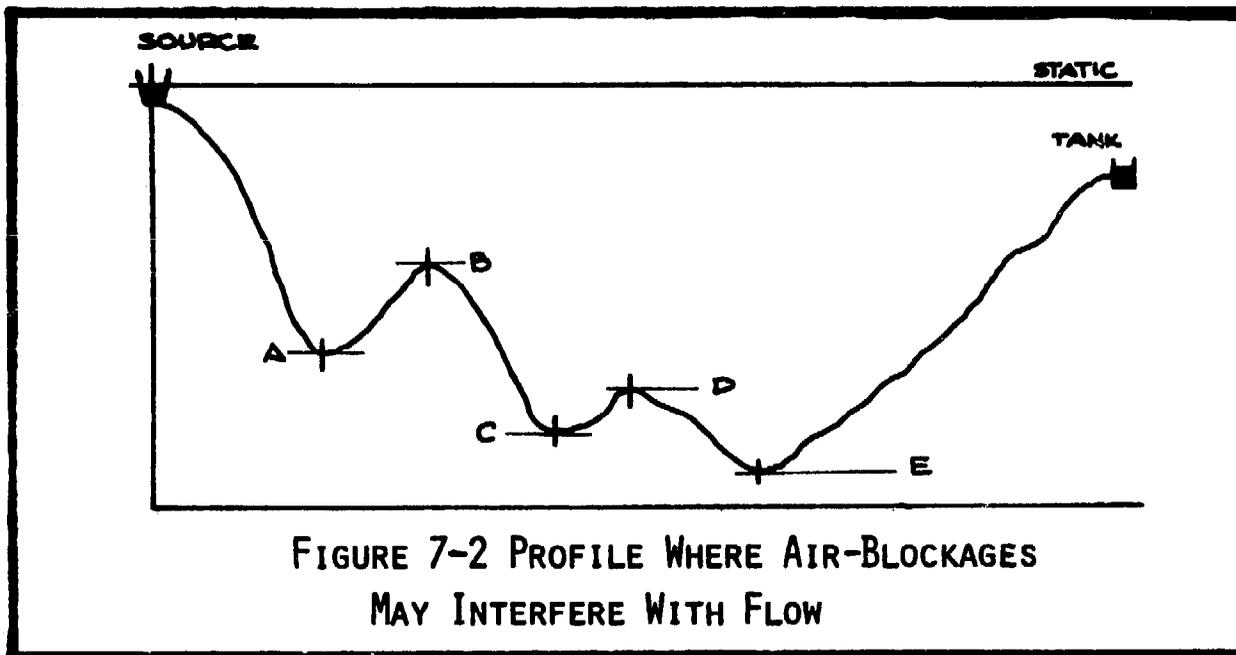
FIGURE 7-2 PROFILE WHERE AIR-BLOCKAGES
