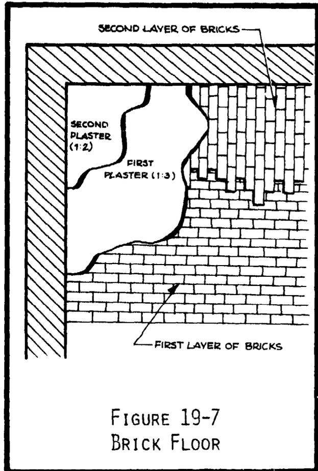
no spatterdash coat needed). As soon as the second plaster coat has set, the tank should be flooded a few centimeters deep (for curing the mortar) for several days. Refer to Figure 19-7.
