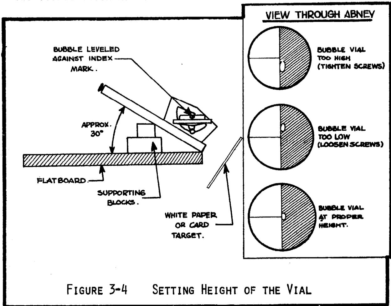
Hold a white card in front of the tube and sight through the instrument. The bubble should be centered on the cross-hair. If it is not, adjust the height of the bubble level by tightening or loosening the mounting screws equal amounts in the same direction. If the bubble appears too low, then lower the level by tightening the screws, and vice versa.
