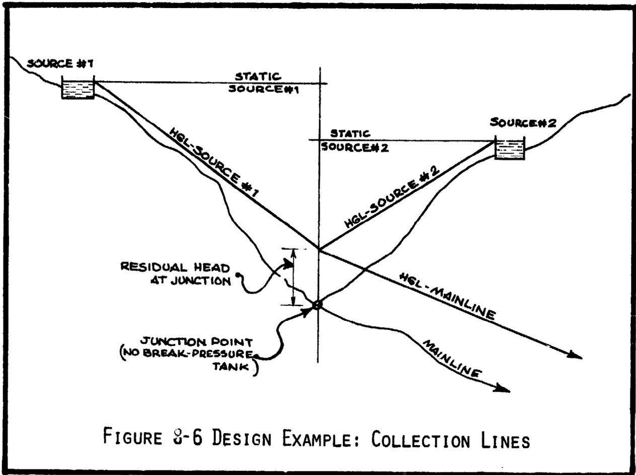
FIGURE 8-6 DESIGN EXAMPLE: COLLECTION LINES
