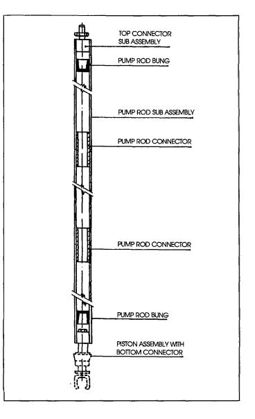
consists of a galvanized steel spindle threaded at both ends. The steel spindle was chosen because of the need to detach the piston assembly from the pump rod to change the valve and seal.
