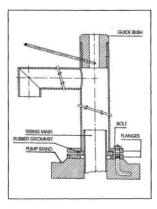
The guide bush is made from a tropical hardwood (sal) soaked in vegetable oil and encased in a sheet metal sleeve to contain swelling. Though the zinc is rapidly removed from the handle by rubbing against the guide bush, this does not lead to corrosion, because of the daily polishing in normal use.
