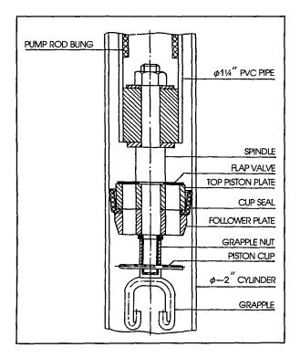
The piston assembly bears the load of the column of water on the upward stroke of the pumping cycle. The rubber flap valve alternately closes on the upstroke to seal the piston ports and opens on the downstroke to let water pass through to repeat the cycle.
