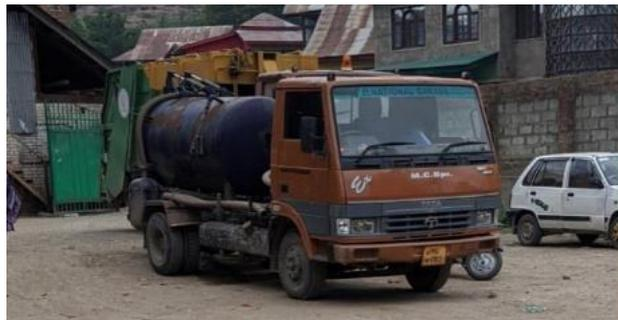
**Figure 3: Govt. operated vacuum tanker of 2,000 L capacity.**
