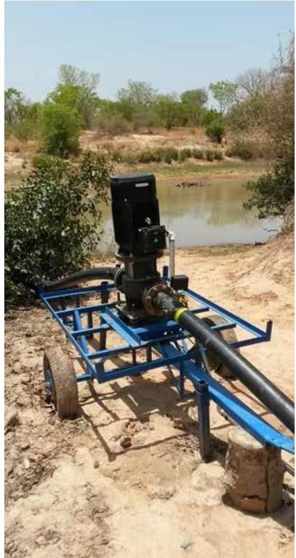
Surface pump on a mobile structure
