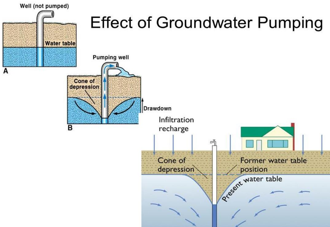
Figure: Effect of Groundwater Pumping
