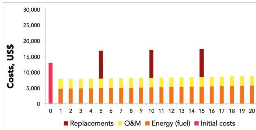
Figure 5. Yearly costs of a diesel-based pumping system.
