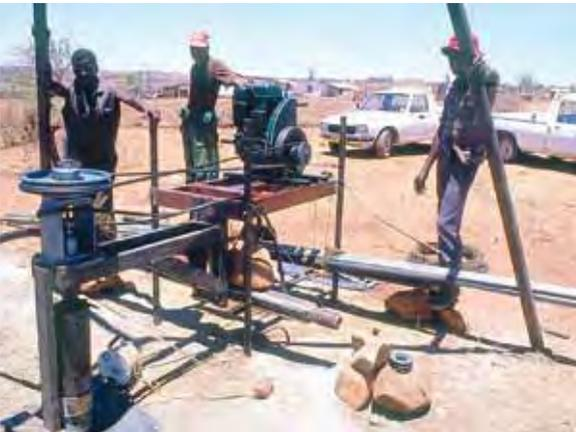
**Figure 17. A test-pumping rig in operation (it consists of a belt-driven mechanical rotary (Mono) pump), Zimbabwe**
