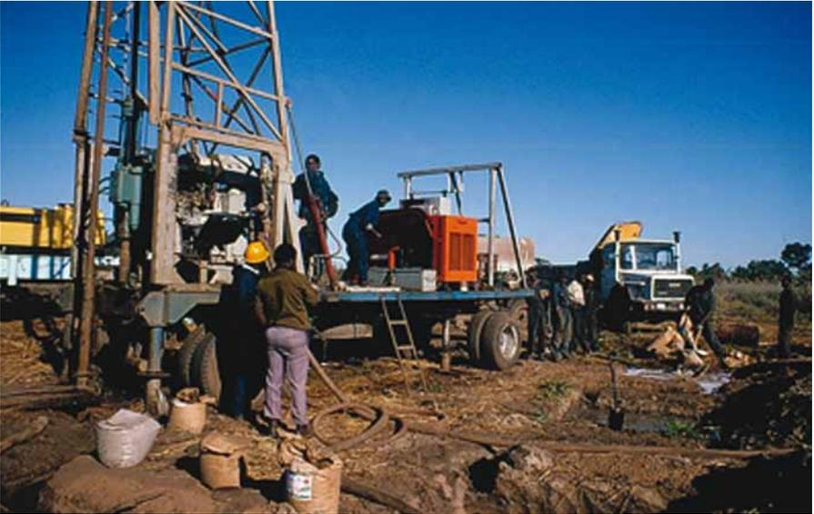
Figure 2. A mud rotary machine working in eastern Zimbabwe, 1996. Note the mud pits dug nearby.
