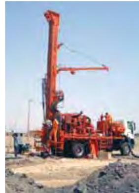
**Figure 7. The Dando Watertec 24 drilling rig**
