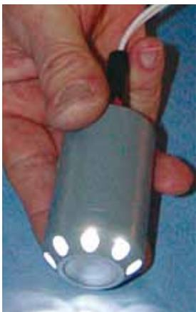
**Figure 19. A CCTV borehole camera**
