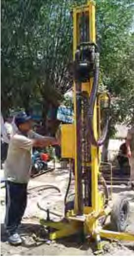
**Figure 5. A PAT 301 drilling rig**
