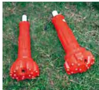
**Figure 9. DTH hammer button bits. The hammer body, into which it slides, is not shown.**
