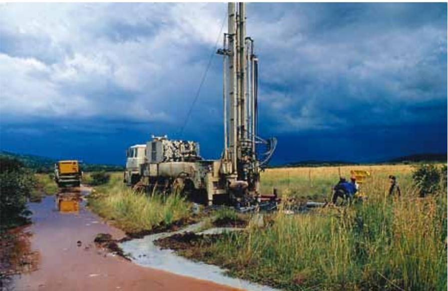
Figure 3. Air rotary machine developing a successful borehole, South Africa, 1989
