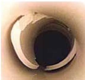
**Figure 18. Casing damage as seen through a CCTV borehole camera**
