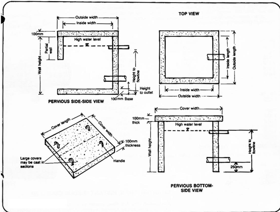
Figure 4: Dimensional plans of pervious side spring box and pervious bottom spring box (courtesy of USAID, 1982, available online at [www.lifewater.org](http://www.lifewater.org)).
