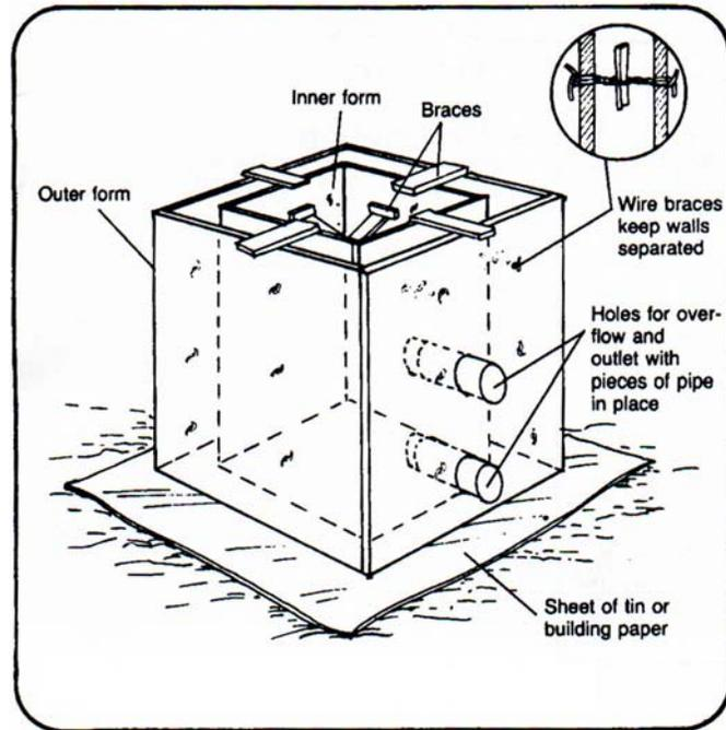
Figure 8: Form for a permeable-bottom spring box.
