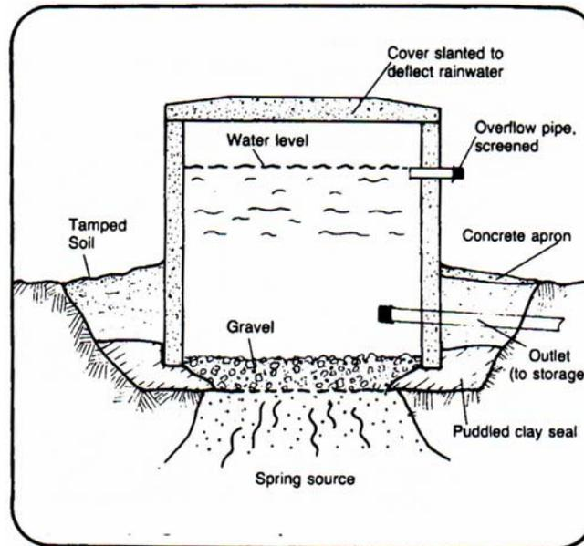
Figure 2: Spring box with permeable bottom for collecting spring water flowing from an opening on level ground (Courtesy of USAID, 1982, available online at [www.lifewater.org](http://www.lifewater.org)).
