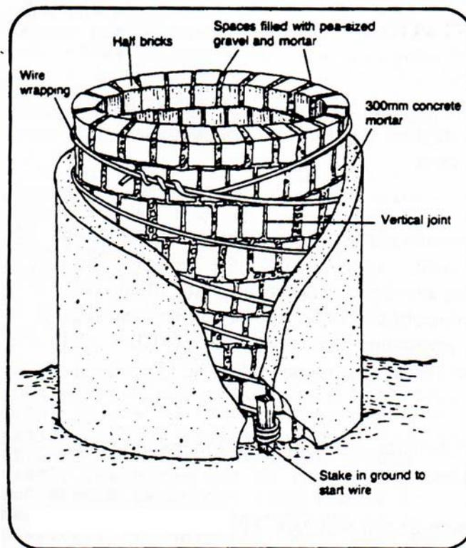
Figure 3: Spring box constructed with brick, wire and cement.
