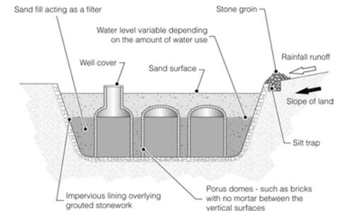
Sand-filled sub-surface tank, Botswana
