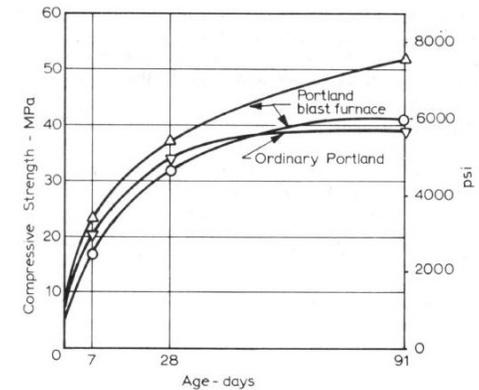
Concrete strength with curing
