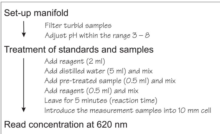
**Figure 6.6** Flow chart of fluoride analysis by complexone method at the range 1–20 mg l<sup>-1</sup> F.
