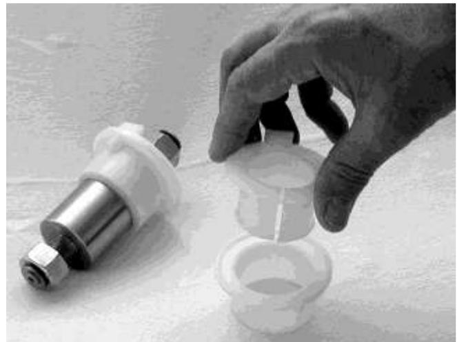
5.5.4 Place all remaining pump components like pump cover and handle parts close to the installation spot and keep the small components like bearing bushes, fulcrum- / hanger pin and all nuts and bolts in the pump head cover.
