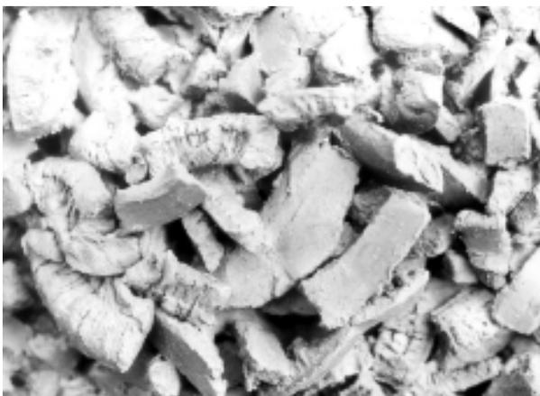
**Figure 2.9** Individual clay cuttings washed to the surface
