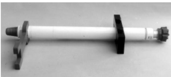
**Figure 3.3** *Down-the-hole hammer – with stripping clamp and spanner*
