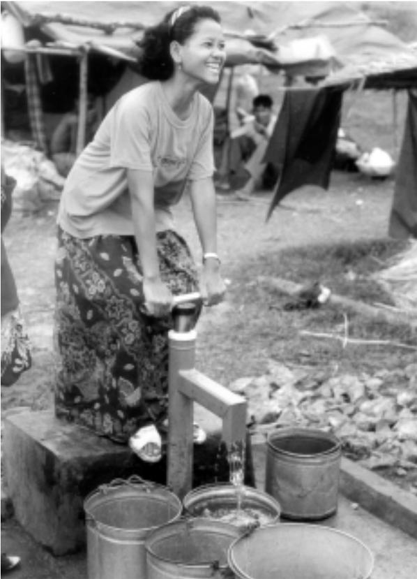
**Figure 6.2** *Direct Acting hand pump*
