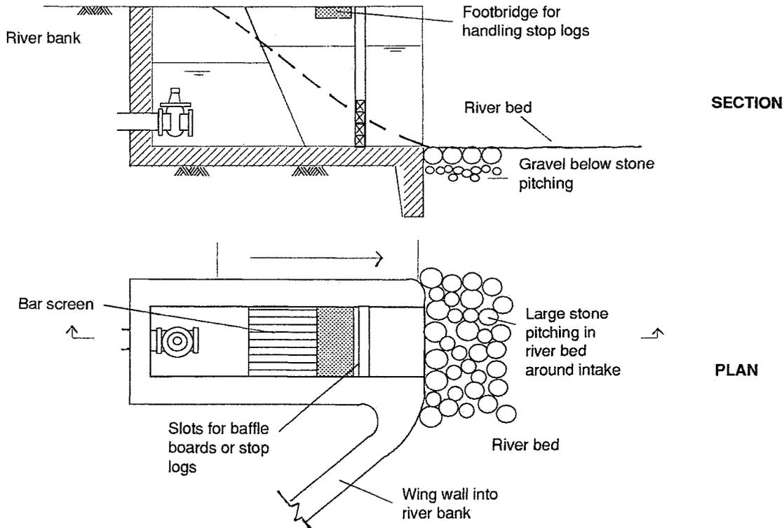
In the side intake the water is abstracted through an intake built in the river bank. The example includes wing walls into the bank and large stone pitching to protect the intake against floods and scour. A duplicate intake may be provided to facilitate maintenance.
