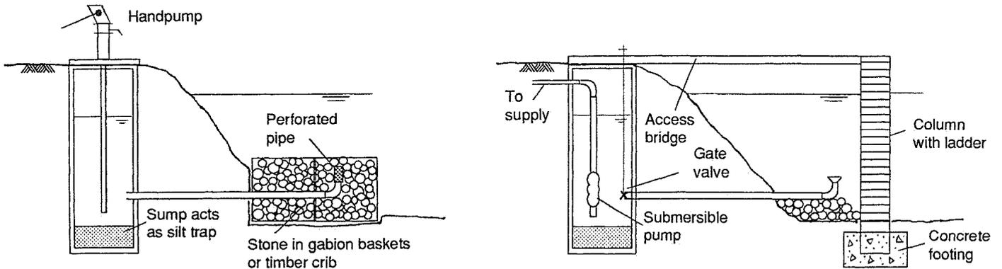
Problems can arise with all of the above intakes if the river bed is unstable (for example, gravel), or the river is very shallow at low flows. It can be difficult to set the intake level to be safe from silting up during floods, but still able to abstract water at low flows. A weir can assist with this (see opposite) or a floating intake can be used.
