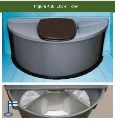
four-compartment composting tank with a lid and a seat with a cover, both made of rigid plastic. Air circulation via the ventilation pipe keeps the composting toilet odourless. The containment system is rotatable so that when one half of the containment is full, a thin layer of soil or compost is sprinkled over the top, and a new compartment is rotated into position. One compartment holds a summer's worth of faeces and bio-waste from a household of four persons.
