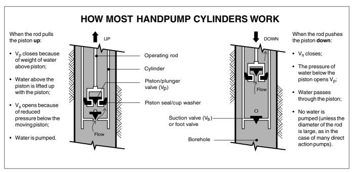
In most handpump cylinders a piston is alternately raised and lowered by a rod (or a string of rods joined together) which is connected to a handle, or sometimes to a flywheel and crank. These pumps are called **reciprocating handpumps.** The figure above illustrates how most cylinders work.
