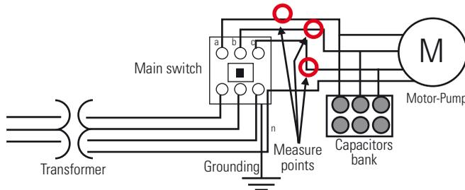
**FIGURE 8:** Measuring the Real Power after the Capacitors Bank
