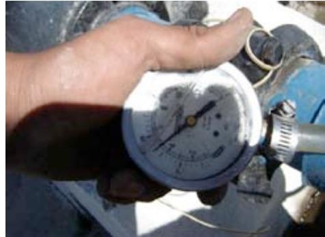
For practical purposes, head load pressure calculations should be expressed in meters of water column (mwc), although the gauges normally have scales in ( $\text{kg}/\text{cm}^2$ ) or (PSI). The equivalence formulas of these units are:
