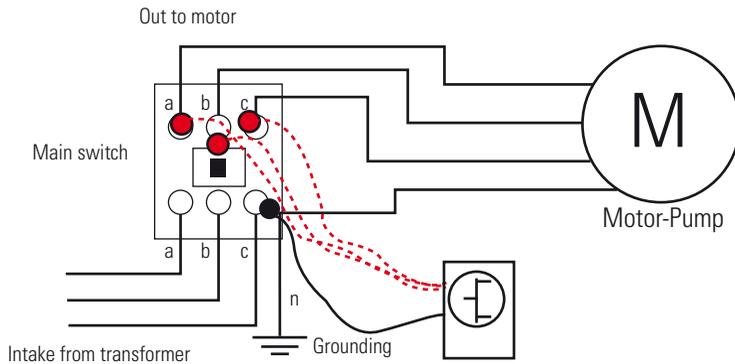
7. The value of the three-phase voltage (V) can be calculated with the average of these three values. Take three readings in each cable to confirm the data. Define a realistic variation range for minimum and maximum acceptable values.
