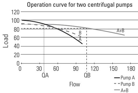
The load capacity equation then supposes that:  $Q_{AB} = Q_A + Q_B$
