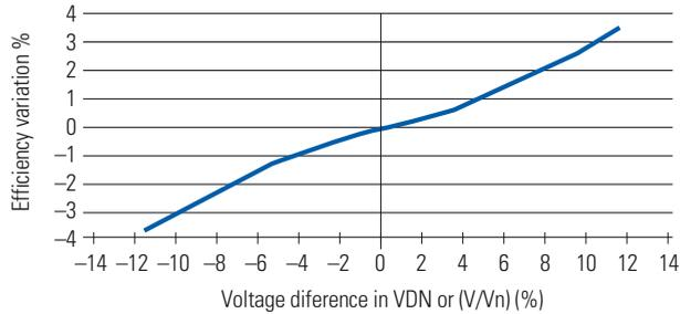
If there is an imbalance in the supply voltage, apply the adjustment to the efficiency according to the curve in Figure 20.
