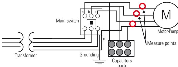
electric motor in evaluation. The second measurement must be upstream of the capacitor. This measurement will describe the effect of the compensation of the PF on the electrical network.
