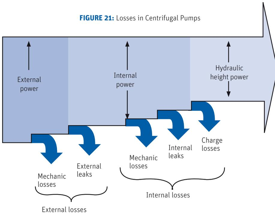
The overall efficiency of the operating pump is then calculated as the total output power  $P_s$  (pressure in the output gauge) divided by the mechanical power absorbed  $P_m$ , identified in Figure 21 as external power. The efficiency formula is as follows:
