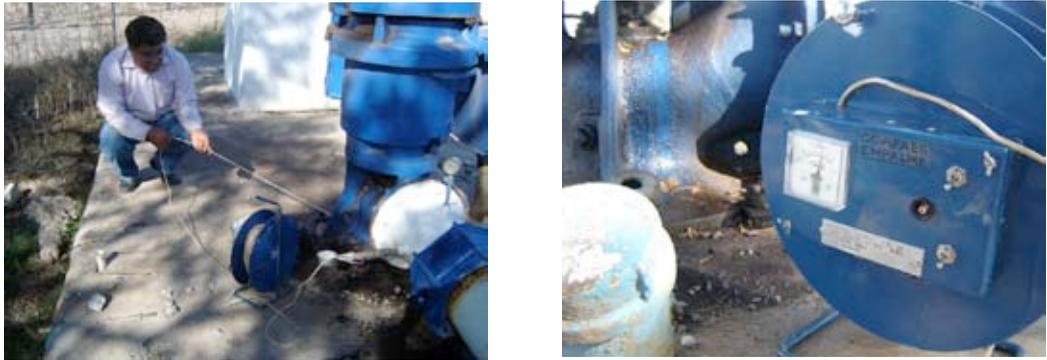
**FIGURE 15:** Measurement of the Dynamic Level of a Low-Level Water Tank
