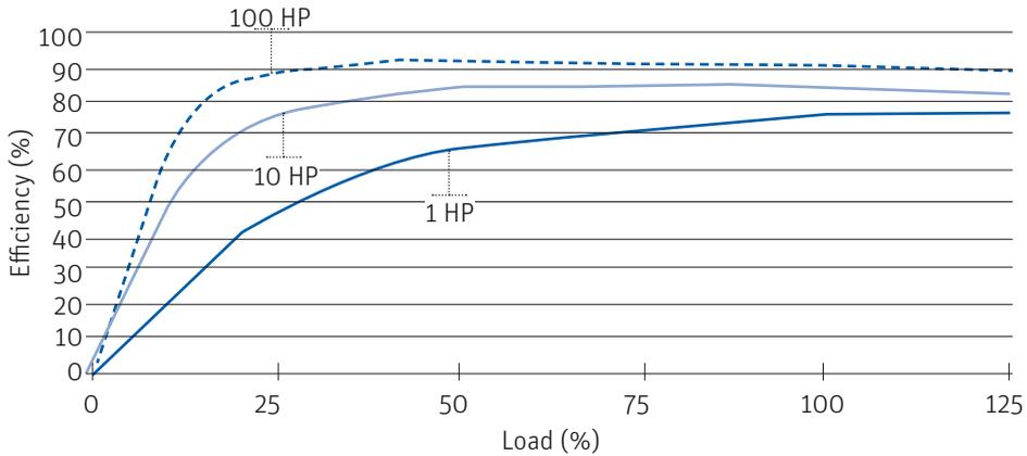
The appropriate motor efficiency curve, identified in Figure 18, is derived from the original design parameters of the motor (HP, RPM, and V). Using the measurement of the active power of the motor, calculate the LF using the following equation:
