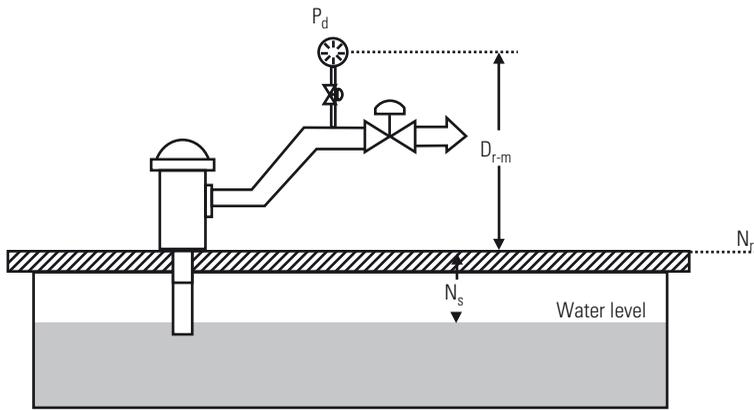
**FIGURE 12:** Measurement of Pressure When Gauges in Suction and Discharge Are Available
