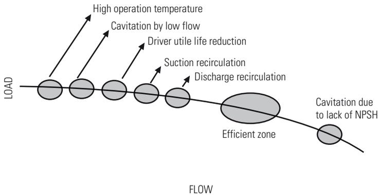
Pumping systems commonly operate at different conditions than those for which they are designed. The causes of this problem include the following:
