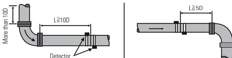
Flow measurement may be carried out in a short period of 15 to 30 minutes. If flow variations are less than  $\pm 5$  percent in the course of a full day, the average flow value is recorded. If the flow fluctuation is greater than this percentage, continuous testing should be carried out for at least 24 hours to establish an average flow value.
