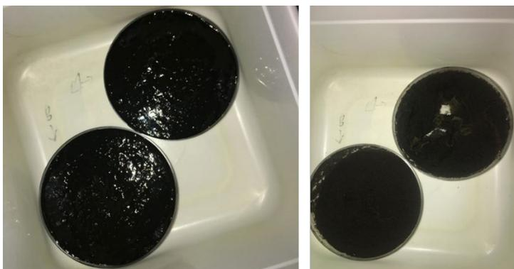
Figure 51. Sludge sample before and after solar drying in sunny conditions (left and right photograph, respectively)
