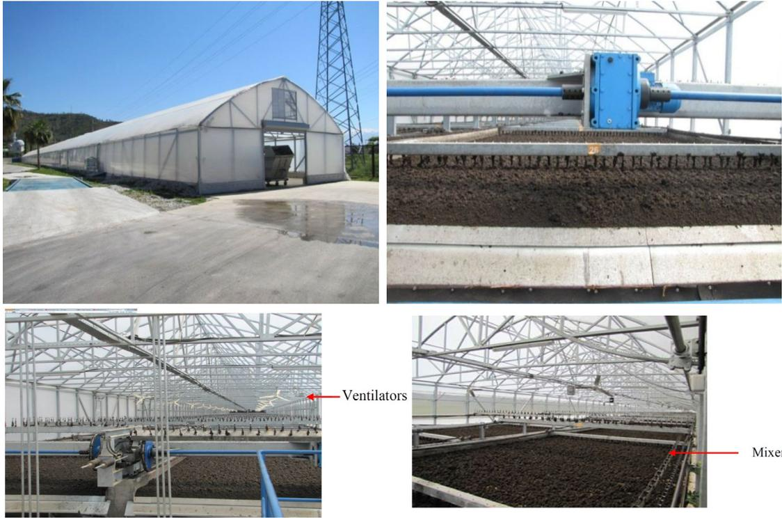
Figure 78. Solar drying greenhouse in Fethiye wastewater treatment plant, Turkey (Kurt, 2014)
