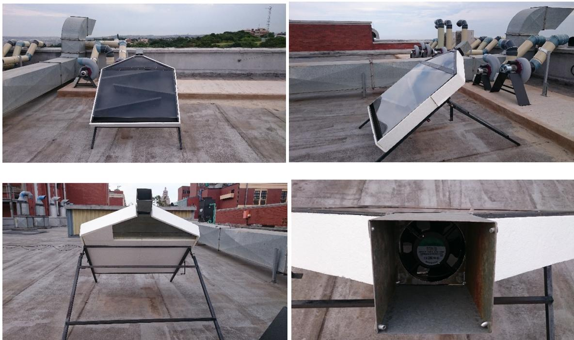
*Figure 92. Photographs of the solar heating chimney*
