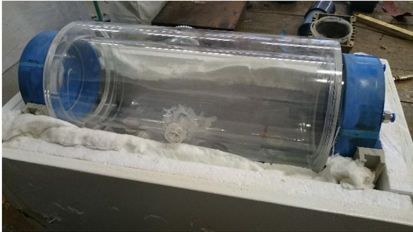
Figure 27. Drying chamber inside the protection box
