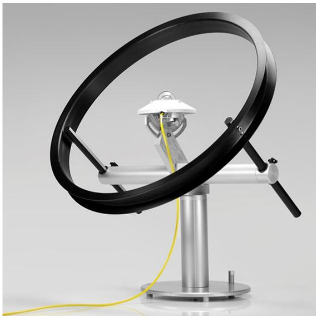
*Figure 7. Shadow band pyranometer*
