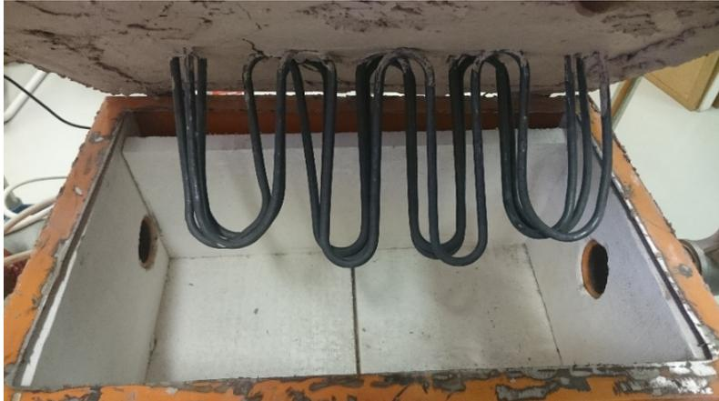
Figure 29. Interior of the air heater
