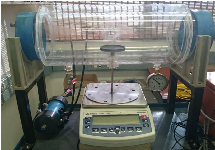
Figure 26. Setup of the sample support in the solar drying rig
