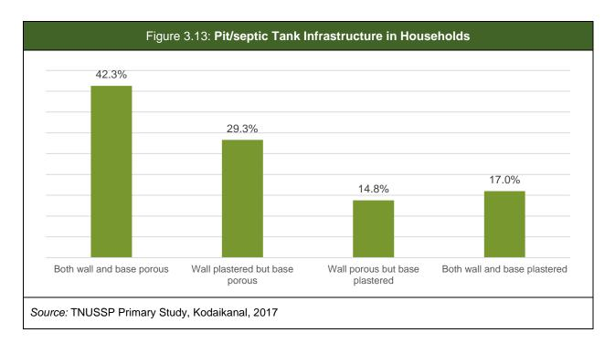
As per WHO standards<sup>13</sup>, it is necessary for a septic tank to be watertight and it should ideally have at the least one partition wall so as to meet the two-chamber criteria.
